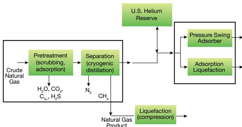
▲ **Figure 5.** Helium production involves a multistep process to recover crude helium from natural gas and then refine it into high-purity helium. Source: (8).
