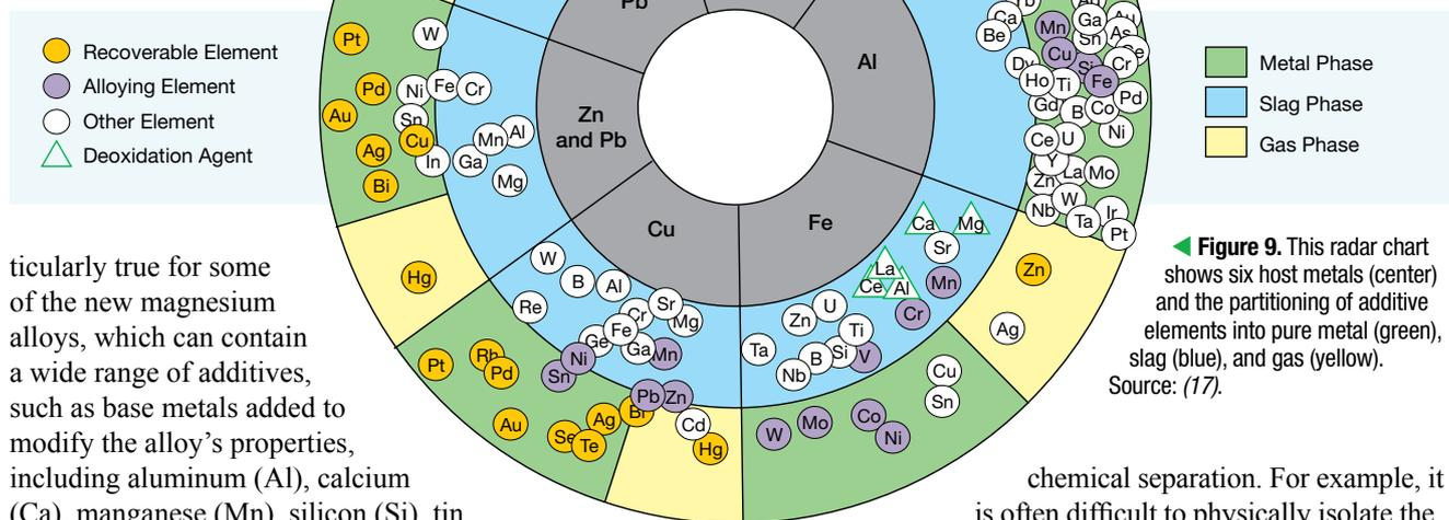
◀ **Figure 9.** This radar chart shows six host metals (center) and the partitioning of additive elements into pure metal (green), slag (blue), and gas (yellow). Source: (17).
